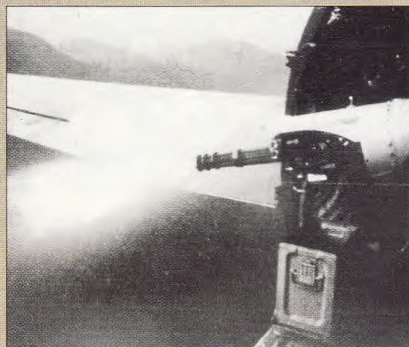
When Miniguns were fired at night, it looked as if a laser gun were being shot from the ship. The weapons' powerful kick would yaw the plane to the left, so while firing the guns, the pilot had to hold right rudder or use differential thrust to stay on target (photo courtesy of Norm Taylor).
