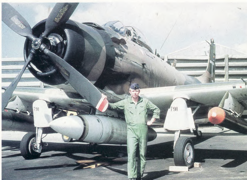
The author with A-1H 139-791. This photo gives an appreciation of the size of the Skyraider. The oil dripping on the 300-gallon centerline tank shows the pilot that this Spad is "alive" and ready to go.
