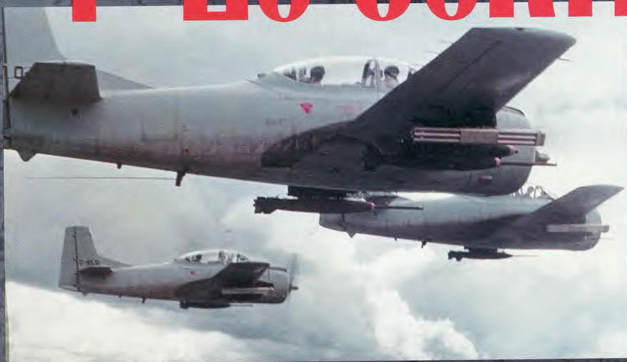
Three Detachment 1 T-28Ds with CBU and Mk 81 or Mk 82 with fuse extensions are on their way to the "customer's" target.
