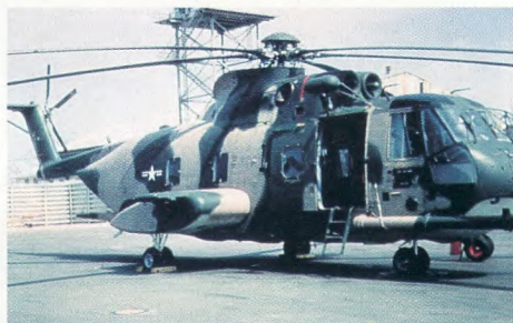
Above: an HH-3E on the ground at Da Nang, South Vietnam. The CH-53 and HH-3E looked very similar. The 3E could be refueled while airborne, it had foam-filled tip tanks that self-sealed when hit, and it had a tail minigun in addition to the two in the waist positions. During the Mayaguez incident, three CH-53s were shot down, and the rest took punishing hits from machine-gun, mortar and grenade rounds (photo by Don Doran, courtesy of Ric Hunter). Left: the Sikorsky CH-53 was the largest heavy-lift helicopter used by the Air Force in the Vietnam War. Along with CH-53s, the HH-3Es provided the only transportation into and out of combat action for Marines on Koh Tang Island (USAF photo, courtesy of Ric Hunter).
