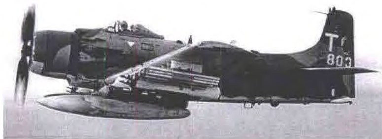
Capt. Buck Buchanan flying A-1H 139-803 over South Vietnam on 5 July 1972. In addition to the normal ordnance load, this Skyraider is carrying 5-inch Zuni rockets "procured" from the USMC A-4 Skyhawk squadron also flying out of BienHoa and 2.75-inch rockets with 17-pound warheads "borrowed" from the U.S. Army Air Cavalry unit at BienHoa.
