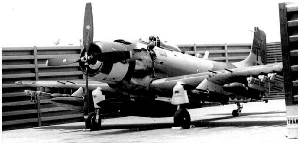
Figure 6 Single-seat A-1H Skyraider s.n 139-780 with typical Sandy SAR weapons load, Da Nang Det. 1 Sandy alert revetment.
