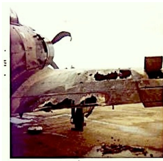
Figure 16 A-1H, s.n. 139-780 battle damage
