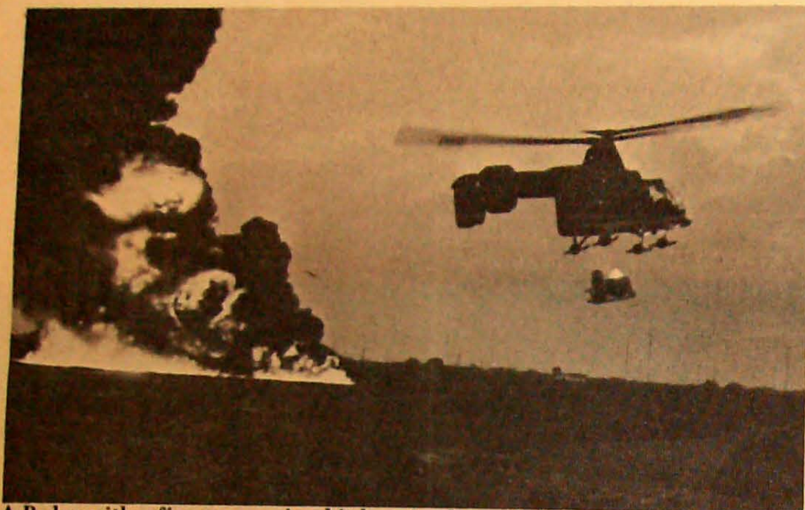
A Pedro with a fire suppression kit hanging beneath it moves into the area of a fire
