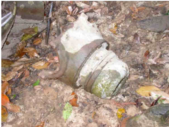
This piece of wreckage is an actuator that moved the tail section control surfaces.
