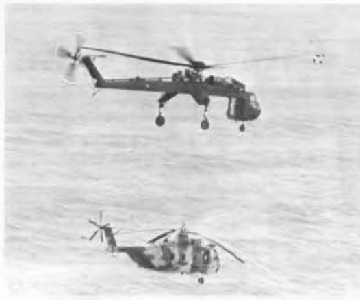
HH-3E helicopter, down in Tonkin Gulf for 16 hours, is lifted by CH-54A Flying Crane and carried to repair base.
