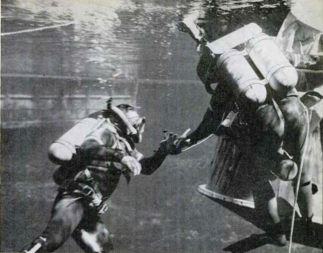
SPACECRAFT RECOVERY is similar. Two-man team attaches floatation device to capsule before inflating it
