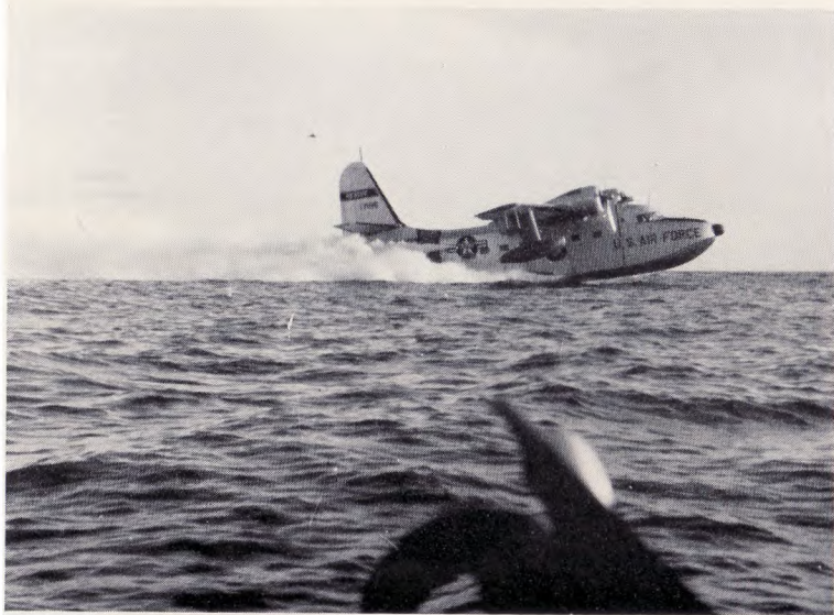
The JATO bottles used to assist take-off in difficult conditions can be seen quite clearly in this picture of a U.S. Air Rescue Service Albatross
