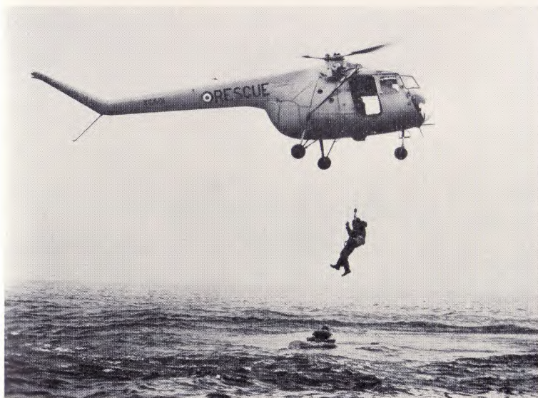
A survivor being winched up to an R.A.F. Sycamore by the single lift method
