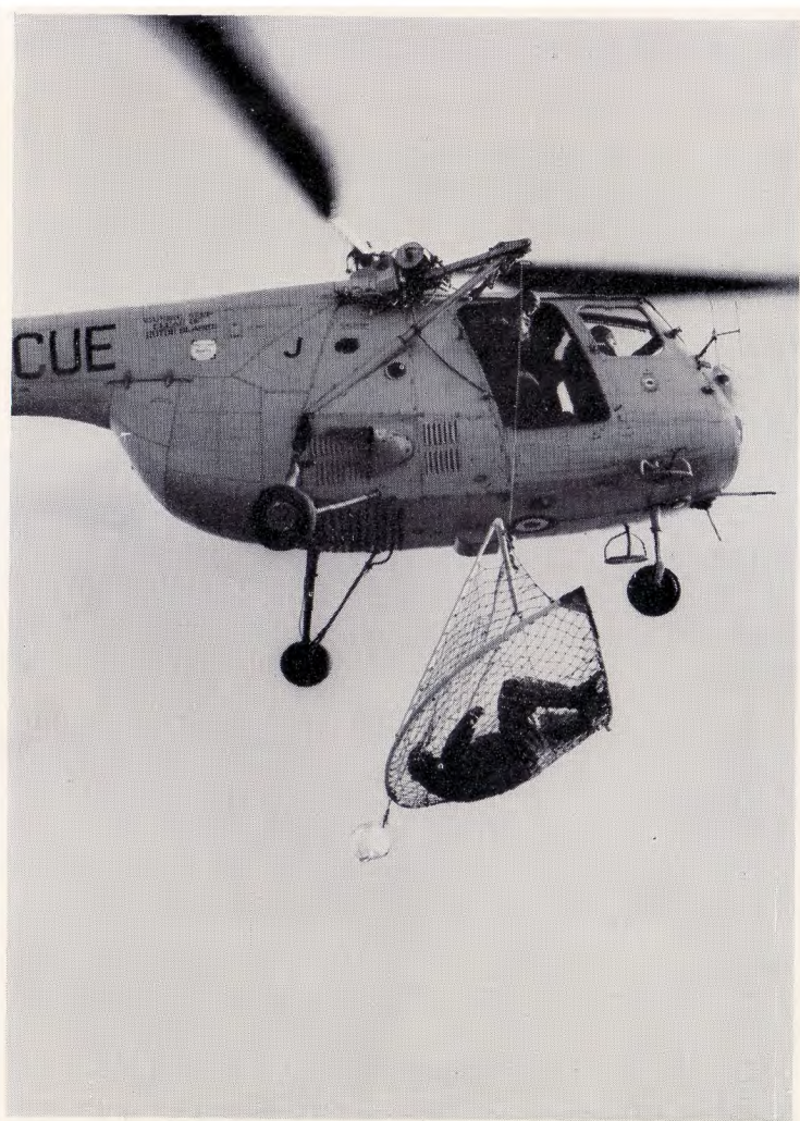
PLATE 5 The scoop net in use. The small white drogue at the back of the net steadies it in the water
