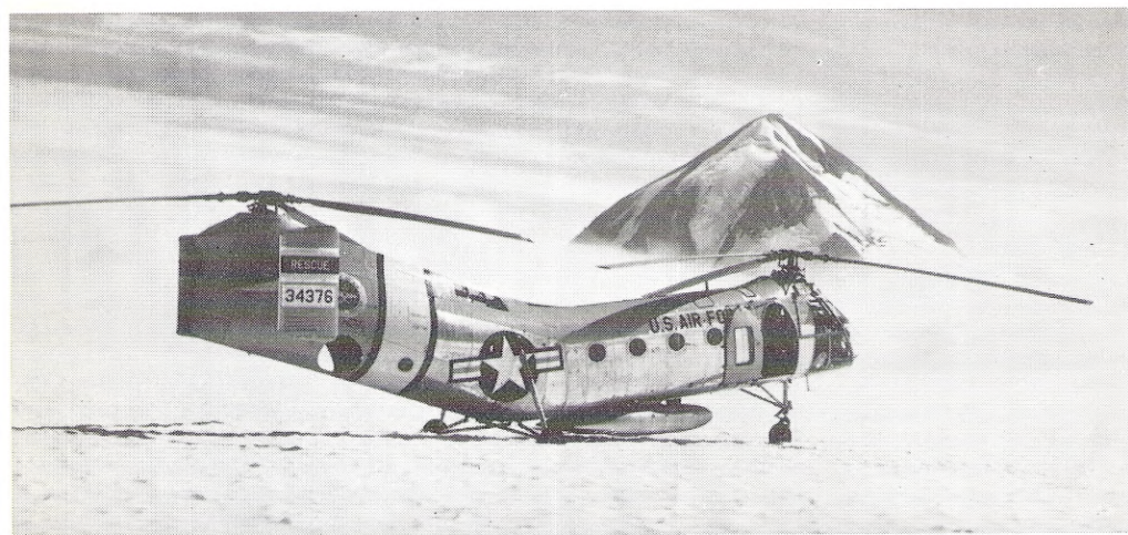
WINTERIZED , range increased, specially modified for Rescue mission, the tandem rotored SH-21B is utilized by squadrons in the north.
