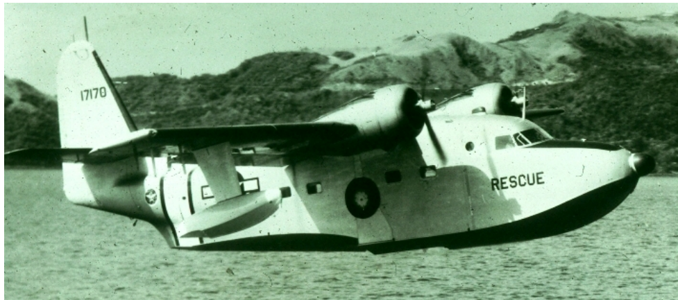
The Grumman HU-16 Albatross is a twin-radial-engined, amphibious flying boat. Originally designated as the SA-16 it was redesignated as the HU-16 in 1962.
