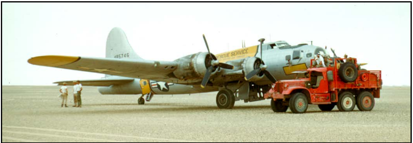
On occasion, landings could be made in the large gravel plain areas to the north of the Rub Al Khali desert. The 6x6 truck takes on a load of gas from the bomb bay tank of SB-17G 485746.
