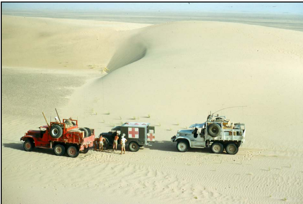
Flight 'D' land rescue vehicles at the northern edge of the Rub Al Khali desert. The 4x4 Dodge ambulance has a flat tire. The 6x6 Diamond T truck on the left carries 800-gallon of truck gas, spare parts, maintenance tools and equipment. The other 6x6 carries 500-gallons of water, food and communication equipment.
