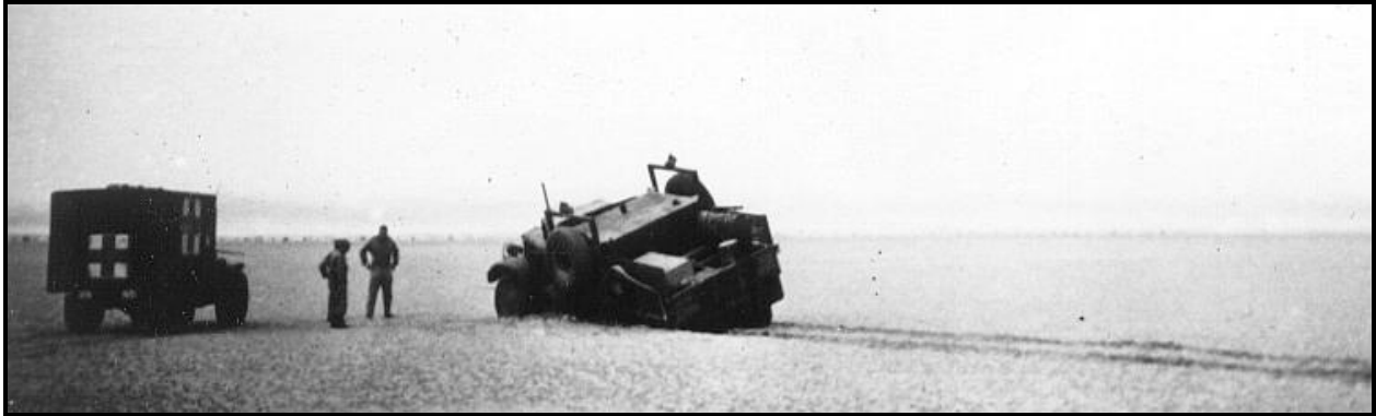
The 6x6 land rescue truck breaks through a hard sun-baked crust into a quagmire that starts to harden like concrete when the air gets to the mud-like mixture. We used the other 6x6 in our effort to pull this truck out of trouble.
