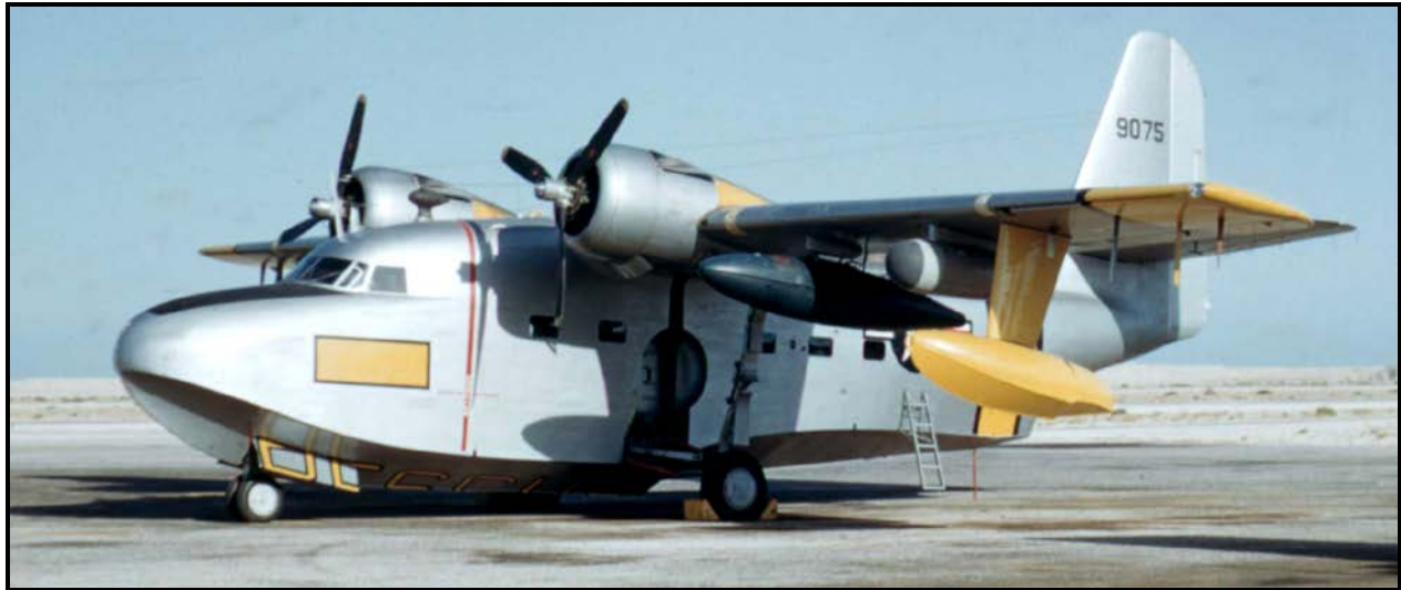
My ship! SA-16A 49-075 on the apron at Dhahran, 1950. This was the 22nd aircraft of this type in the Air Force inventory, and the first to go overseas. Notice the AN/APS 31 radar pod located just inboard of the left wing float. Later models had this radar fitted into the bow of the aircraft.
