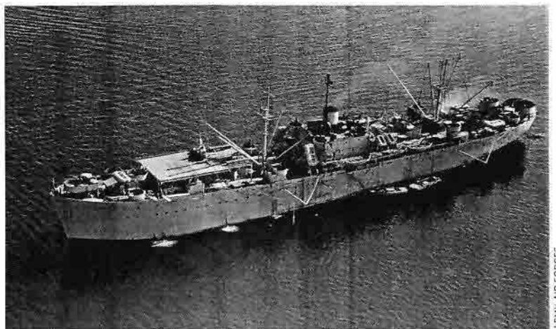
For the wounded on Luzon in 1945, the Sikorsky R-6A transport (opposite) doubled as an ambulance. The helicopters were stationed on aircraft repair ships outfitted with 40- by 72-foot landing decks (above).
